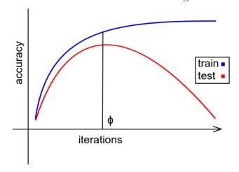
The accuracy of the model on both the training and the test set are presented for various numbers of iterations. The point  $\Phi$  indicates the iteration from which the red graph starts to decrease again.
